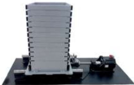
Figure 2. Fixable laminar shear box installed on the table
