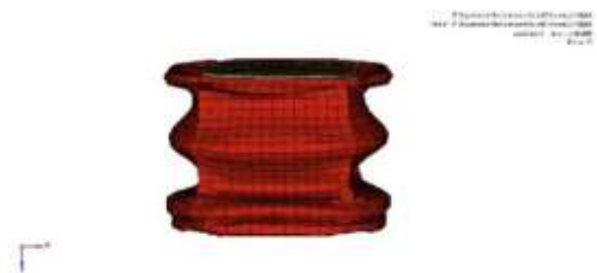
Figure 12. Quasi-static simulation results of square tube with foam aluminum filler
