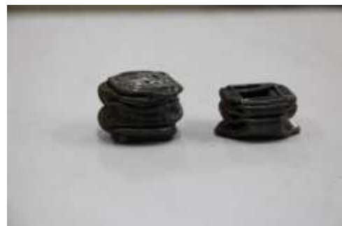
Figure 5. Comparison of compression test results between square and square tubes filled with foam aluminum
