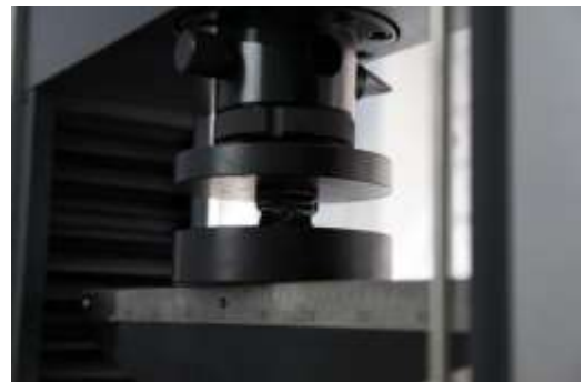
Figure 4. Quasi-static compression result of hollow square tube
