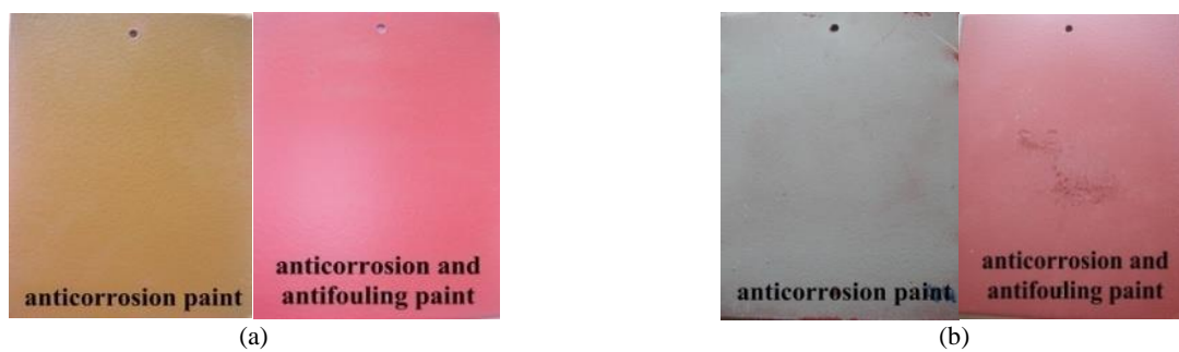
Figure 5. Photograph of (a) AC and AF paints A and (b) AC and AF paints B before exposure
