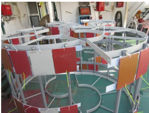
Figure 2. The test rack of specimens for submerged piles of Mandara Bali highway
