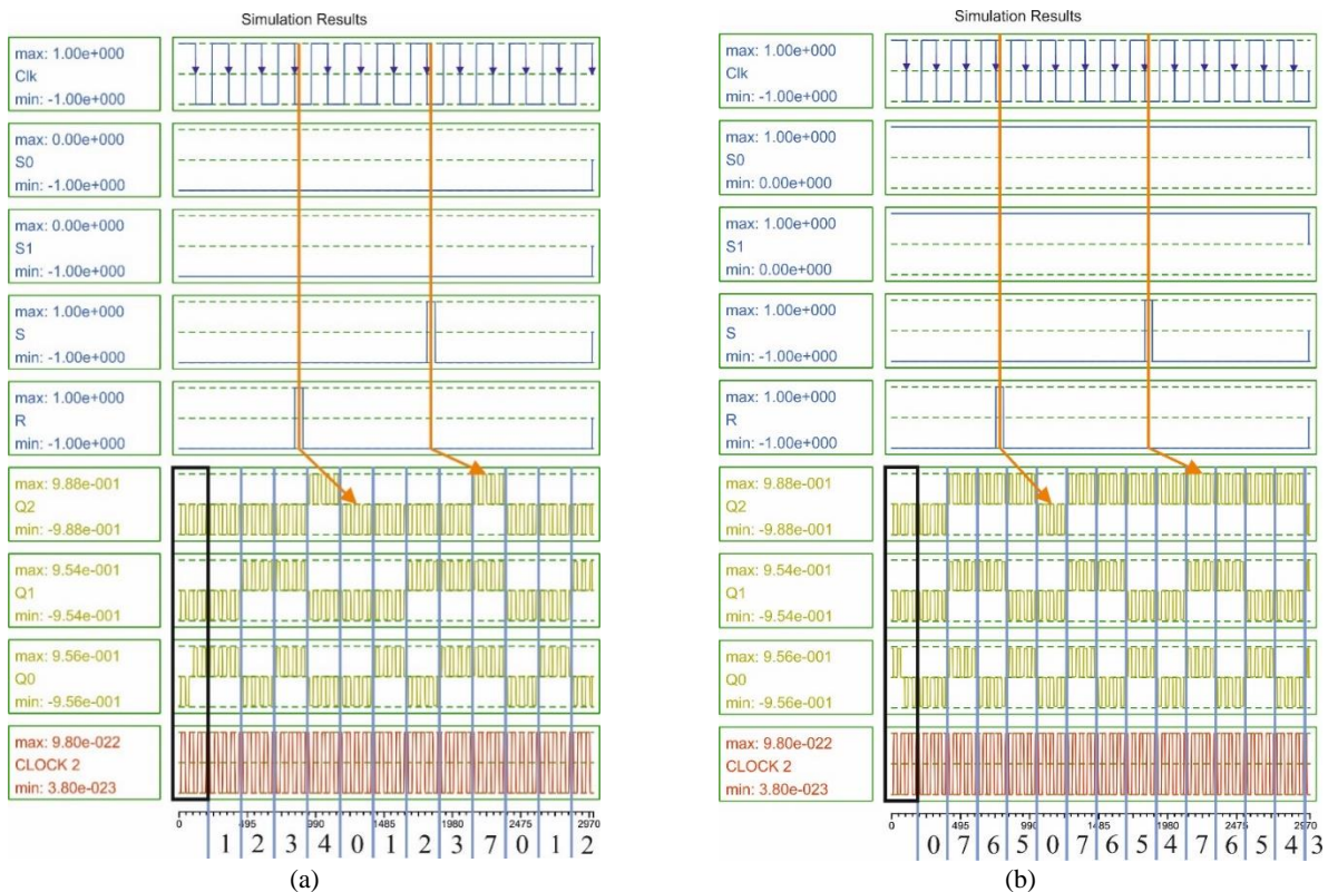
Figure 9. Output waveforms of proposed bidirectional counter with set and reset abilities (a) up direction; (b) down direction
