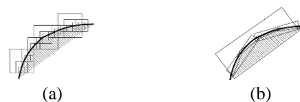
Figure 1. The basic elements located along smooth curves: (a) wavelet versus (b) contourlet transform [23]
