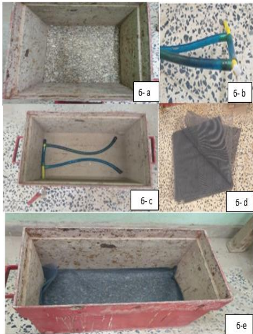
Figure 6. Steps of preparation of soil model loading test
