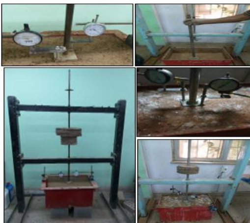
Figure 7. Performing loading on gypseous soil pressure
