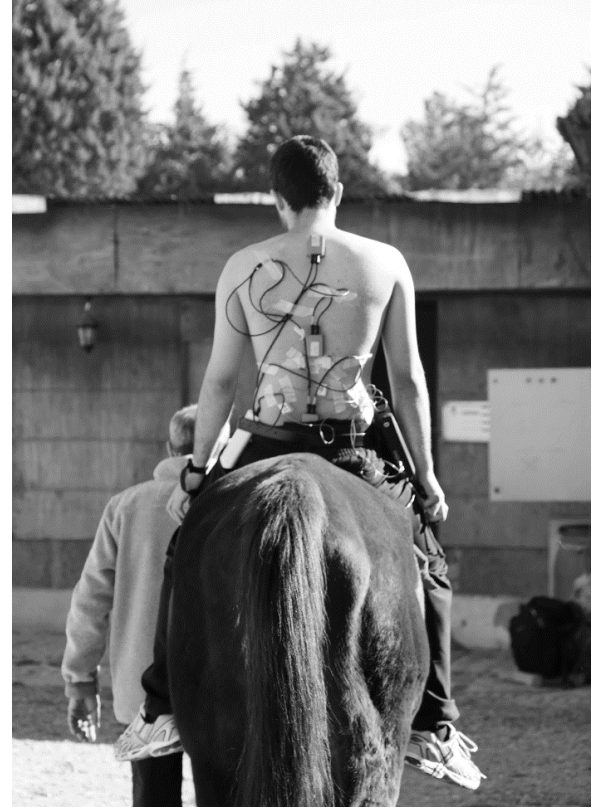
Figure 3. Test subject with IMU and EMG sensors attached
