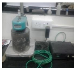
Figure 1. Shrinkage Cone Test setup
