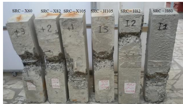
Figure 5. Ultimate yielding mode and failure of experimental specimens
