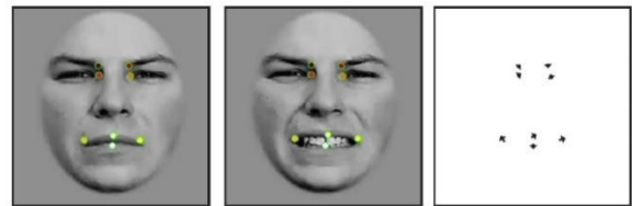
Figure 9. left & middle: two consecutive frames of the movie with designated fiducial points. right: vectors of displacements of fiducial points
