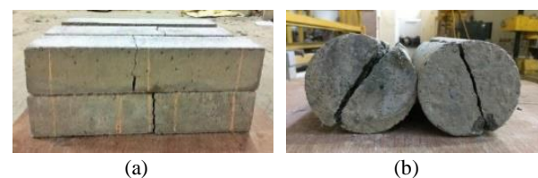
Figure 7. Failure samples after testing (a) flexural strength (b) split tensile strength
