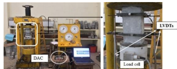
Figure 5. Test setup for concrete stress strain relationship under uniaxial compression loading
