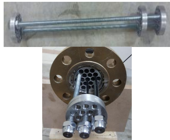
Figure 3. Fixture for positioning sensors at the end of the shock tube
