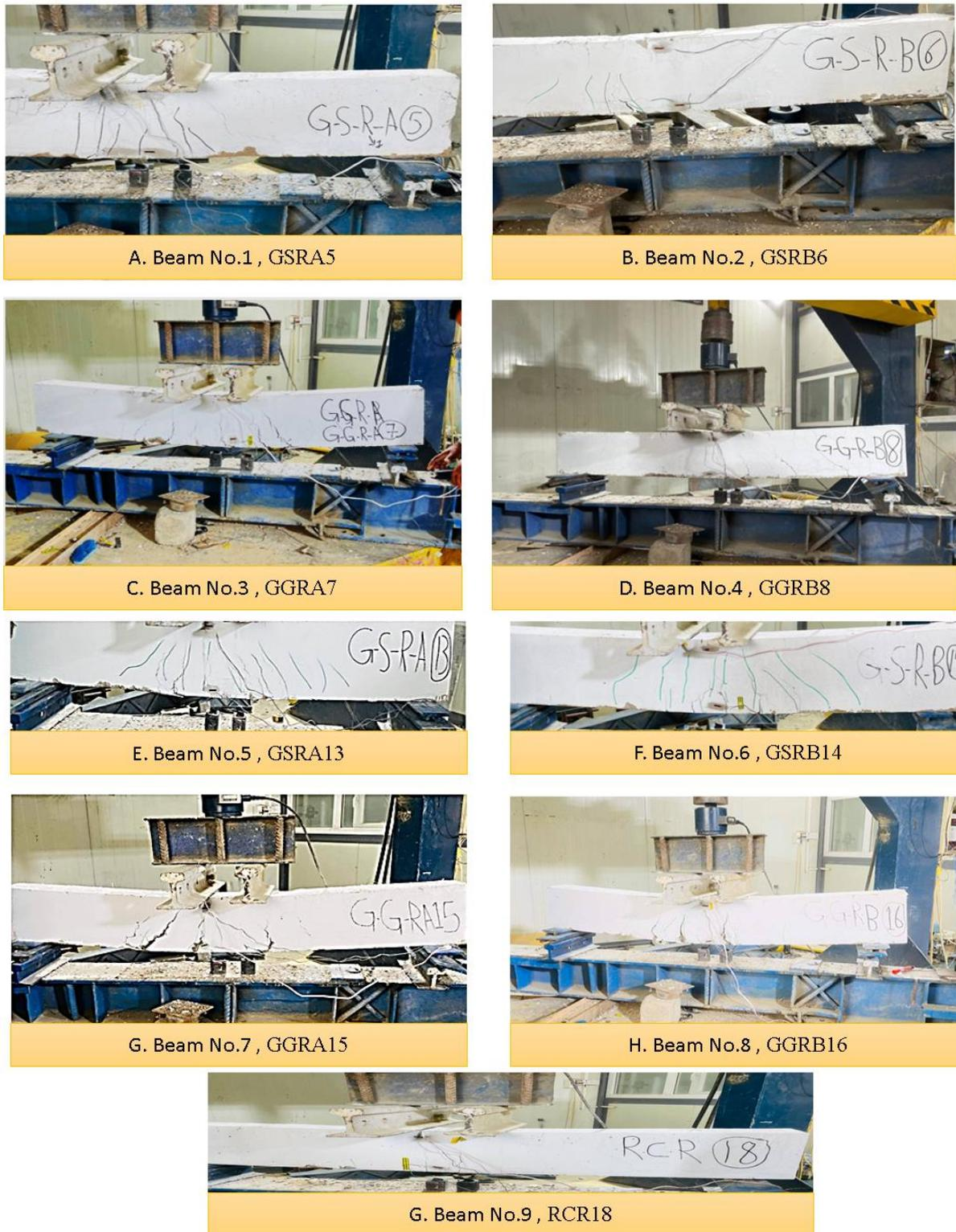
**Figure 11.** Crack patterns for all tested beams
