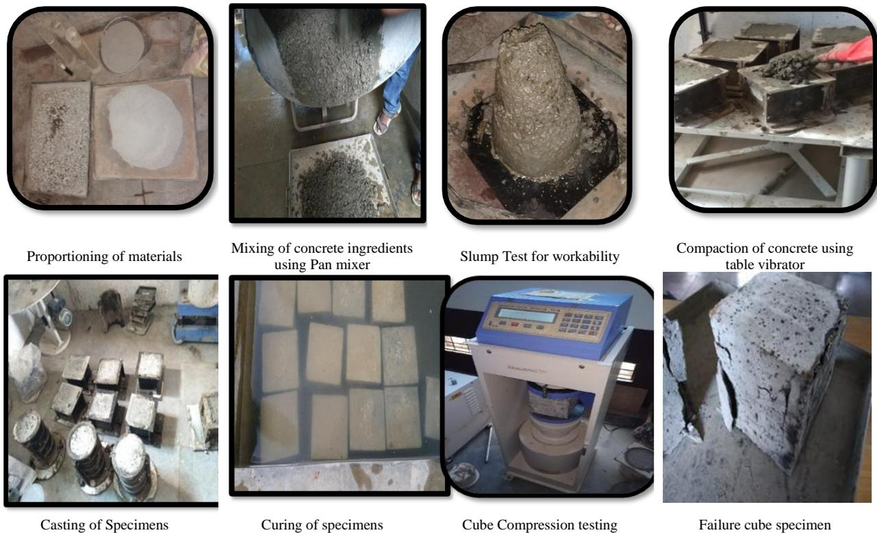
**Figure 10.** Salient process involved in the experimental program
