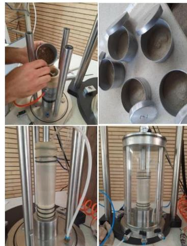
**Figure 6.** Sample preparation in Triaxial device
