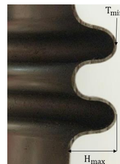
Figure 2. Maximum convolution height and minimum thickness in the top point of bellows congress
