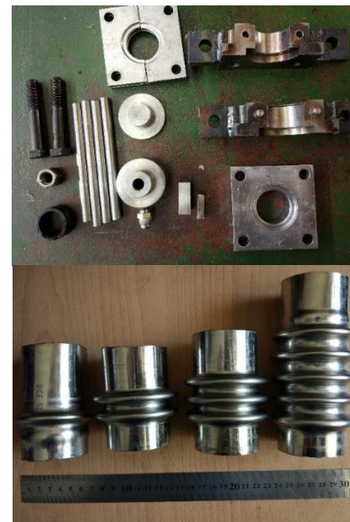
Figure 1. The die set and some of the metallic bellows manufactured by the hydroforming process
