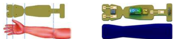
Figure 4. (a) Anatomy correlation between human arm and exosuit base structure in EVA foam, (b) Exosuit with all hardware attached and fabric sleeve-mitten to fit together user arm with exosuit
