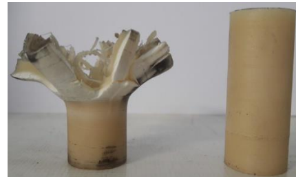
Figure 6. The general view of a projectile before and after impact
