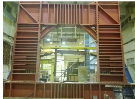
Figure 2. View of frame reaction of experimental tests
