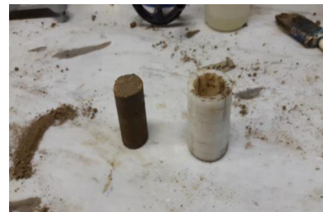
Figure 1. Cylindrical container for single axial compressive test
