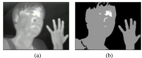
Figure 8. (a) Thermal image, (b) image result using both TOTSU and t_{THER}
