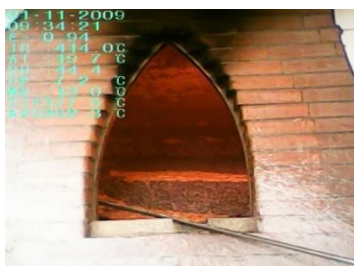
Figure 4. Temperature measurements with IR thermometer for different parts of ovens: (a) Sangak, and (b) Barbari
