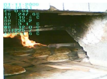
Figure 4. Temperature measurements with IR thermometer for different parts of ovens: (a) Sangak, and (b) Barbari
