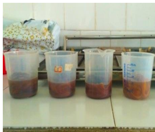
Figure 2. Alkali treatment of fibers
