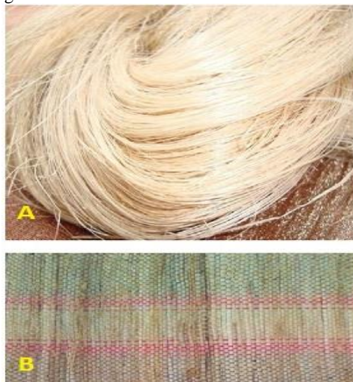
Figure 1. A) Raw banana fiber, B) Woven banana fiber mat
