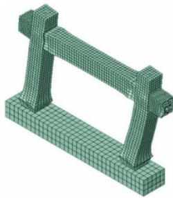
Figure 34. Failure mode primary frame (frame is not retrofitted) in shear
