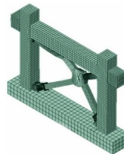
Figure 31. Failure mode of braced frame model NO .1- diagonal member buckling
