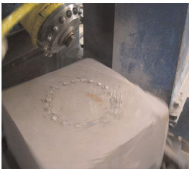
Figure 1. Single-row insert workpiece used to run the indentation test [11]
