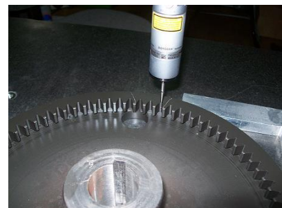
Figure 8. Measurement of wear from tooth profile with CMM device
