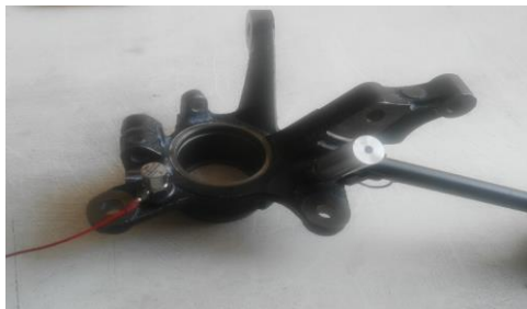
Figure 2. Hammer and accelerometer positions
