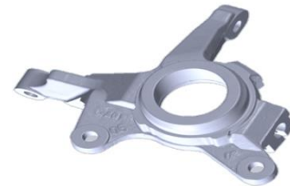
Figure 3. CAD model of automotive steering knuckle by utilizing CMM data
