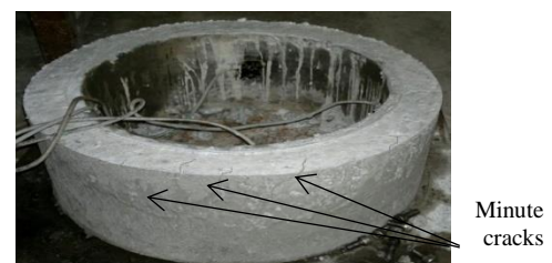
Figure 8. Crack development in Mix CFS4 after 14 days during Ring Shrinkage test
