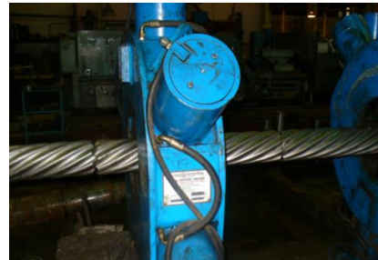
Figure 5. Adjustment of the modules turn angle \phi
