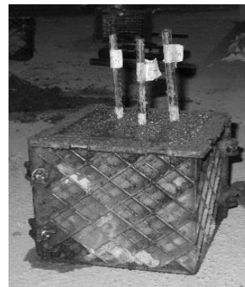
Figure 1. Reinforced concrete during molding and the location of steel bars
