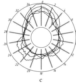
**Figure 2.** Circular plots of deviation of cross sections of the inner cylindrical surface after the following process operations: a) – rough boring; b) – semi-finish boring; c) – finish boring using a special head
