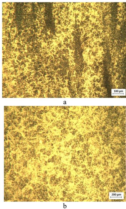
**Figure 4.** Steel microstructure of bearing 22316
