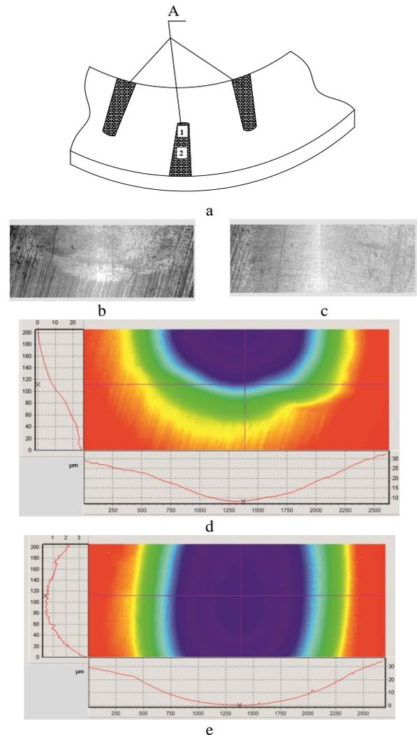
**Figure 3.** Investigation scheme of the inner surface of the outer bearing ring 22316- a, fragments of wear grooves - b, c and corresponding profile charts - d, e; 1,2 – points of surface analysis; A - false brinelling;
