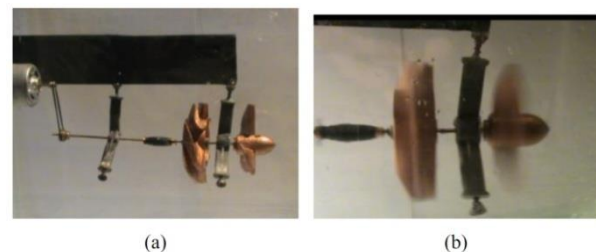
Figure 3. a) Test setup with a thin flexible slab that has black color and b) high speed rotation test in air at 3000 rpm
