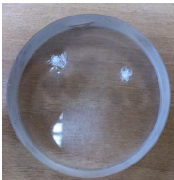
Figure 1. Image of glass sample surface after 5 hits of indenter (general view)
