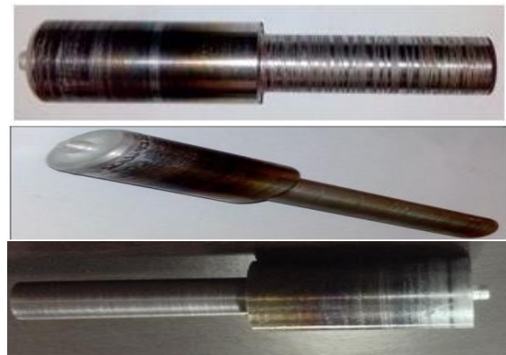
Figure 1. Tool round type with shoulder diameters of 17 mm, 20 mm and 22 mm
