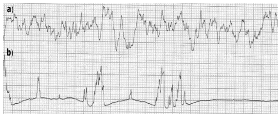
Figure 5. Surface profiles of MCrAlY coating a) Sample A (as-sprayed) b) Sample B (polished).
