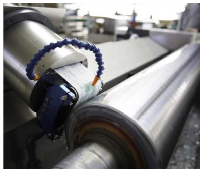
Figure 5. Finishing the printing cylinder by finish star machine
