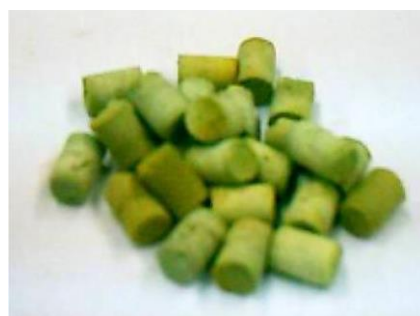
Figure 2. Picture of the extruded form of the catalyst number 1
