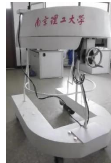
Figure 1. The new gait rehabilitation training robot
