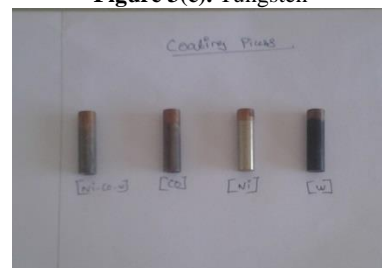
Figure 3(d). Aluminium Specimens used for coating Ni Co W
