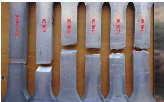
Figure 12. Tensile failed samples (rotational rate \omega /welding speed v ).
