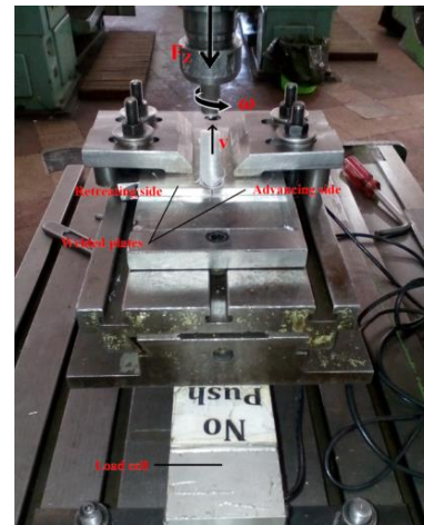
Figure 1. Photograph of FSW that includes conventional nomenclature
