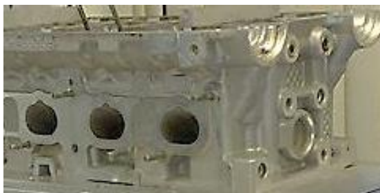
Figure 7. Cylinder head on flow bench equipment
