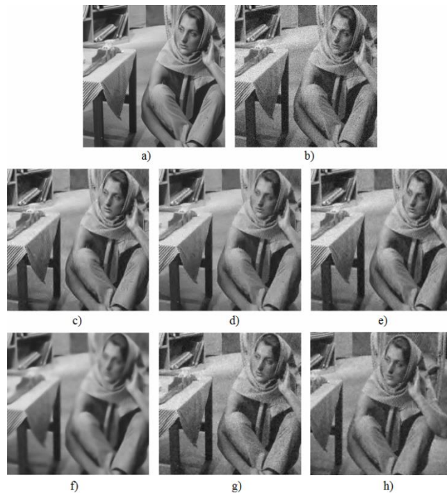
Figure 6. visual results of different denoising methods and proposed algorithm for image Barbara: a) original image, b) the noisy image with \sigma = 30 , c) denoised by ProbShrink, d) denoised by BLS-GSM, e) denoised by SUREbivariate f) denoised by NL-means, g) denoised by TV model, h) denoised by proposed method
