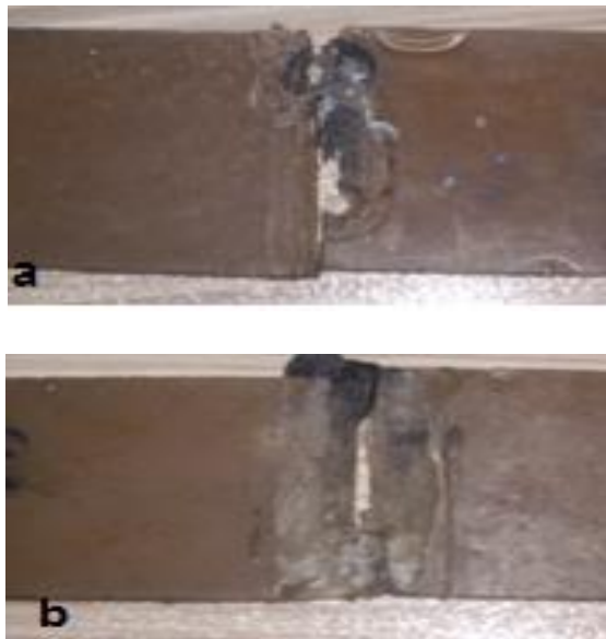
Figure 2. Low quality welds at (a) high welding speed (b) low welding speed
