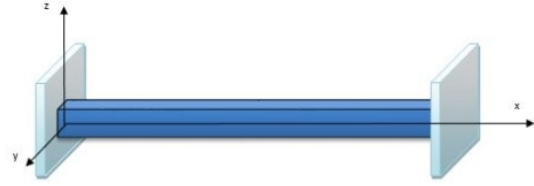
Figure 1. Schematic view of micro-beam with both ends clamped
