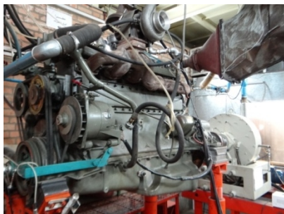
Figure 3. Experimental turbocharged CNG engine on test bed.
