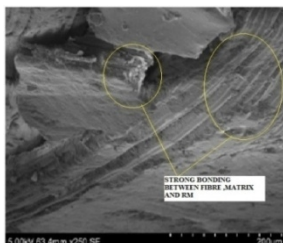
Figure 4(e). SEM studies on the effect of 10% wt Redmud on the flexural strength of 30% wt banana fiber untreated composites
