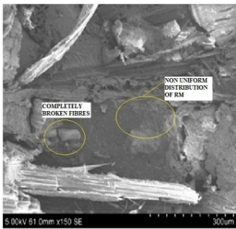
Figure 5(a). SEM studies on the effect of 10% wt Redmud on the Tensile strength of 30% wt NaOH treated banana fiber composites
