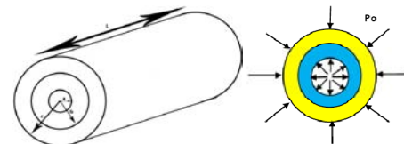
Figure 17. Two-layer cylinder under pressure; prospective and cross section.
