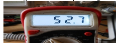
Figure 29. DC Output voltage is measured using multimeter
