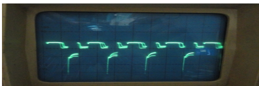
Figure 26. Transformer primary voltage ( V_p )
