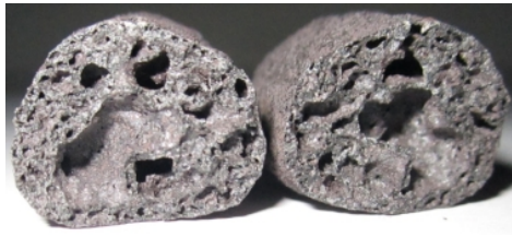
Figure 7. F2 sample sintered at 1100°C with non-homogeneous porosities
