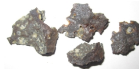
Figure 5. The pressed and sintered (at 1100°C) samples of B1 and B2, the melted appearance was observed
