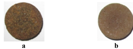
Figure 4. The pressed and sintered (at 1100°C) samples of (a) A1 (b)A2, no evidence of foaming was observed on the surface.
