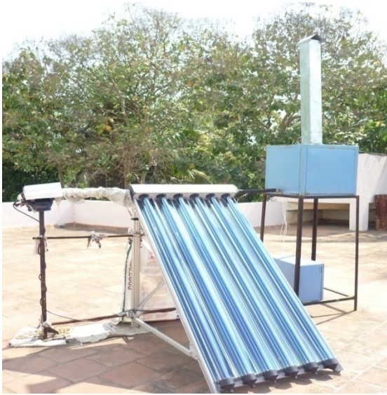
Figure 2. Photograph of the solar drier consisting of drying chamber, evacuated tube collector, blower motor and chimney
