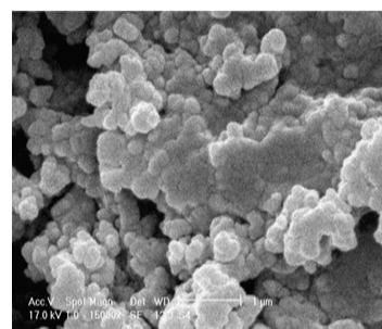
Figure 1. Scanning electron micrograph of PANi Prepared in aqueous media
