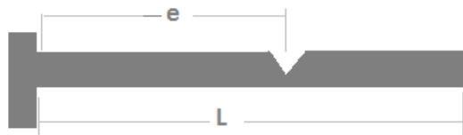
Figure 1. Timoshenko beam with a single-sided open crack.
